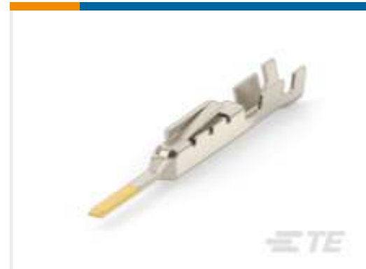
TE Part #1318112-1 Contact: Component To Wire ; 5A, 28-18 wire size, gold plated
