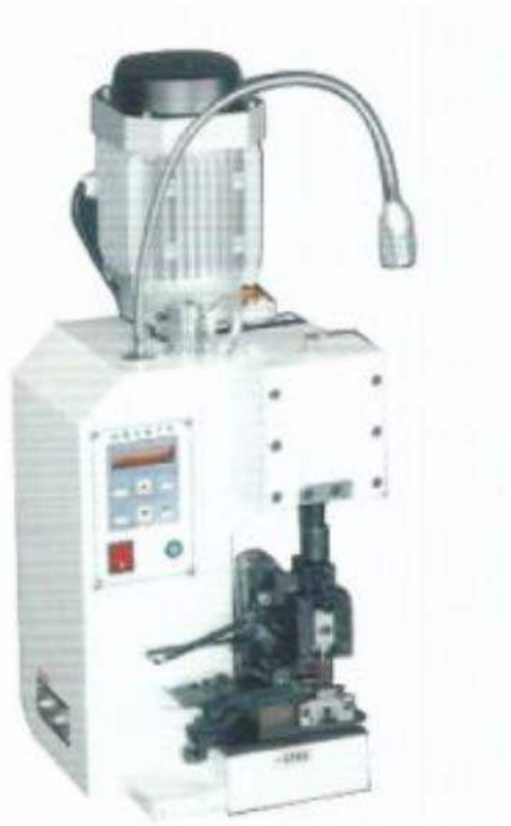
SEMI-AUTOMATED CRIMP MACHINE SHOWN WITH APPLICATOR
