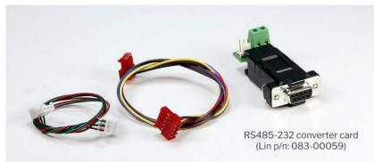
3-Pin to 3-Pin cable for communication 5-Pin to 5-Pin cable for Encoder connection
