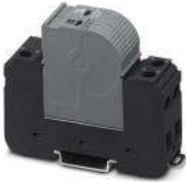
Pluggable type 2 arrester (surge arrester) for 1-phase current supply networks with separate N and PE (3-conductor system: L1, N, PE). Overall width: 24 mm.
