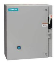
Non-reversing motor starter Size 2 1/2 Three phase full voltage Solid-state overload relay OLRelay amp range 25-100A 190-220/220-240V 50/60HZ coil Combination type 100A circuit breaker Enclosure NEMA type 1 Indoor general purpose use Standard width enclosure
