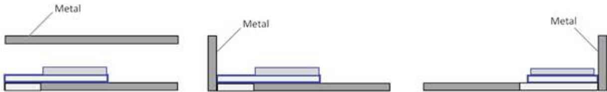
Fig 5-4. Not recommended location in Z plane
