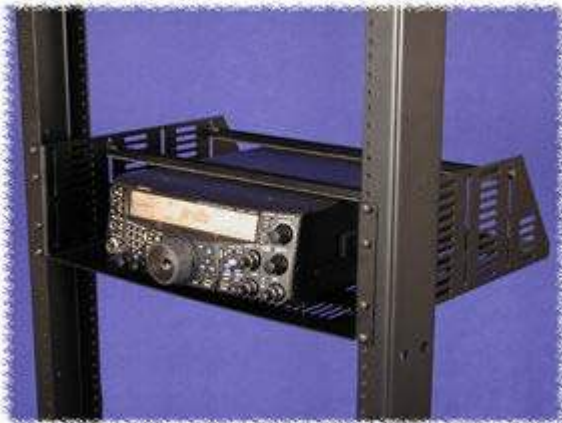
Example of clamped equipment (in this case 10.5" wide)
