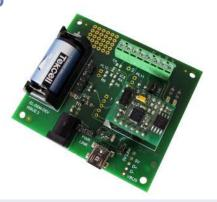
The EL-OEM-TEST is a board designed to assist in development of circuits using the EL-OEM-3 data logger.
