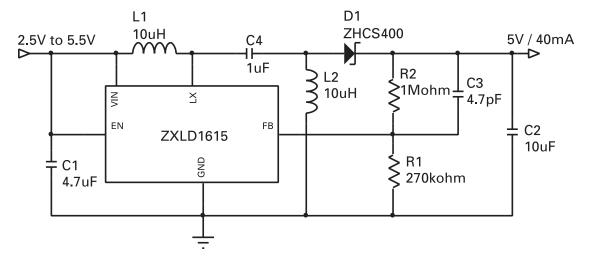
1 Cell Li-Ion to 5V Sepic Converter
