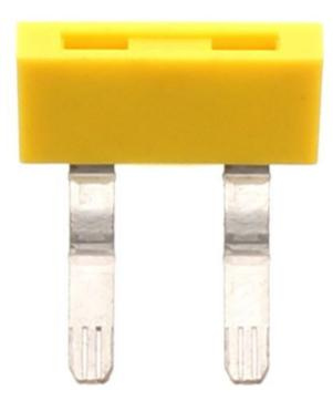
External insulated cross-connector, No. of poles: 2, Mounting type: Plug in, Width: 16.1 mm, Rated current: 27 A; Colour: Yellow
