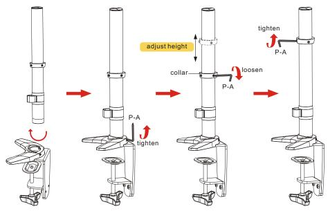
Insert the pole (B) into the desk clamp (C) and tighten the screws using 3mm Allen Key (P-A). To adjust monitor height, first loosen collar screws using 3mm Allen Key (P-A), then set the collar at a desired position and tighten the collar screws using 3mm Allen Key (P-A).
