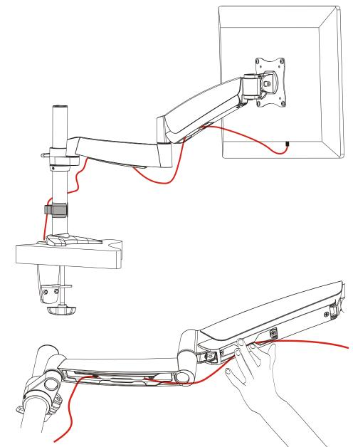
Connect the cables to the display, and press the cable cover inward to route the cables through the space.
