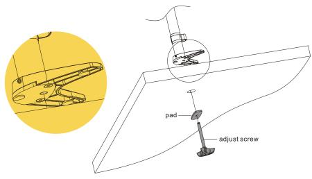
Insert the adjust screw into the base plate through the hole and pad (P-F) as shown above. Then tighten the adjust screw to hold the mount securely.
