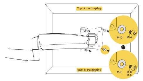
Choose appropriate screws and washers according to the type of your display, and then attach the adapter bracket assembly onto the back of the display, and tighten the screws using a Philips screwdriver.
