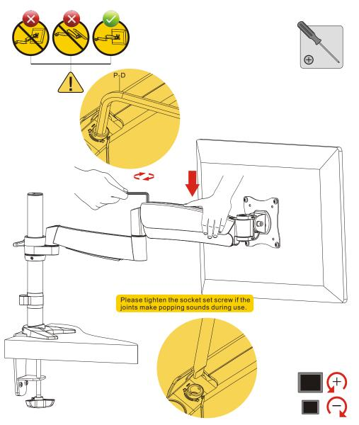
To change the factory preset tension, first apply the force with the forearm and make sure that the arm is level, then using a 6mm Allen Key (P-D), slightly loosen or tighten the adjustment screw as necessary.
