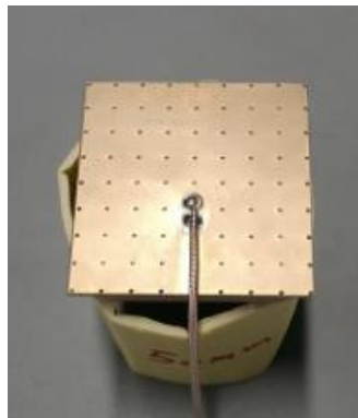
Ground above antenna
