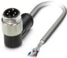
Bus system cable, DeviceNet, 5-position, PUR halogen-free, Gray RAL 7001, Plug angled 7/8"-16UNF, on Free cable end, Cable length: 2 m
