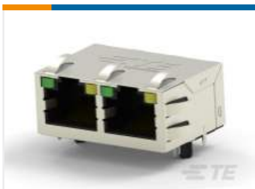
TE Part #5-2337994-3 RJ45 JACK MAG. POE 10/100 LED 1X2 INV.
