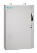
Non-reversing motor starter Size 0 Three phase full voltage Solid-state overload relay OLRelay amp range 0.25-1A 24VAC 50-60HZ coil Combination type 30Amp non-fusible disconnect Encl NEMA type 4X 316 S-steel Water/dust tight non-corrosive Extra-wide enclosure
