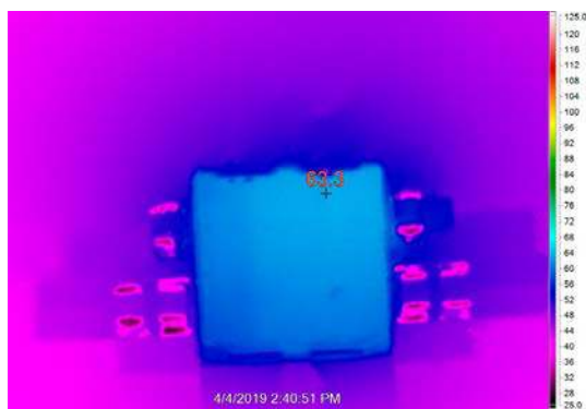
Figure 11. Thermal at V_{IN} = 48V , V_{OUT0} = 1.0V , I_{OUT0} = 25A , V_{OUT1} = 1.0V , I_{OUT1} = 25A , T_A = 25^\circ C , No Airflow
