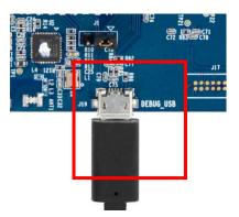
2) Connect the other end of the USB cable to the USB port on your workstation.
