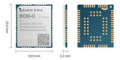
BC95-G is a high-performance NB-IoT module which supports multiple frequency bands of B1/B3/B8/B5/B20/B28 with extremely low power consumption. The ultra-compact 23.6 mm × 19.9 mm × 2.2 mm profile makes it a perfect choice for size sensitive applications. Designed to be compatible with Quectel GSM/GPRS M95 module and NB-IoT BC95 module in the compact and unified form factor, it provides a flexible and scalable platform for migrating from GSM/GPRS to NB-IoT networks.
