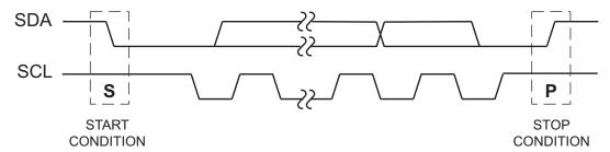
Figure 7. Stop and Start Conditions
