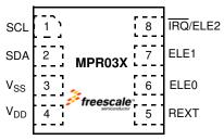
Figure 3. Package Pinouts
