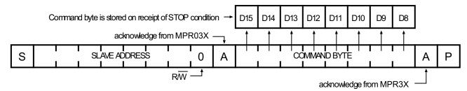
Figure 10. Command Byte Received
