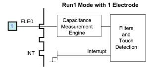
Figure 14. Electrode/Pad Connections in Run Mode
