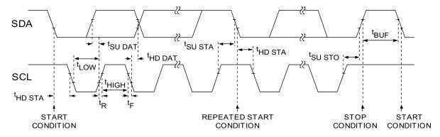
Figure 5. Wire Serial Interface Timing Details
