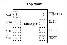
Figure 1. Pin Connections
