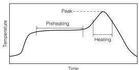
For soldering (Example : Sn/Pb)
