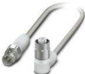
Sensor/Actuator cable, 4-position, PP-EPDM halogen-free, Gray RAL 7035, Plug straight M12, A-coded, on Socket angled M12, A-coded, Cable length: 1.5 m, Hygienic design, With high-grade steel knurl
