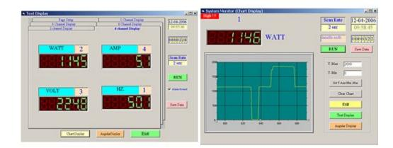
The images above show the software which isused to analyse data and is supplied with the power meter. It can show 4 measurement values at a time and the graphic display can easily storedata over an extended period to be analysed later.
