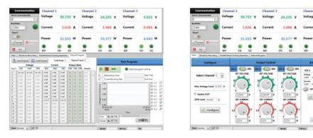
PC software is provided for front panel emulation, generating and executing test sequences or logging measurement data without the need to write source code.
