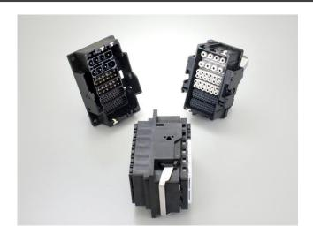
JAE has developed the KN06 Series, a rectangular single-engagement lever locking modular connector. This connector series was developed primarily to be used for large-equipment, such as semiconductor-manufacturing equipment and industrial equipment requiring multi-pole wiring.
