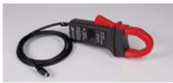
DC600 5 A to 600 A DC; 5 A to 400 A, DC/AC Accuracy \pm 1A \pm 2%, 5A to 400A; \pm 1A \pm 3%, 400 A to 600 A DC Size: 7.68" x 2.6" x 1.34" for conductors up to 1.18" diameter
