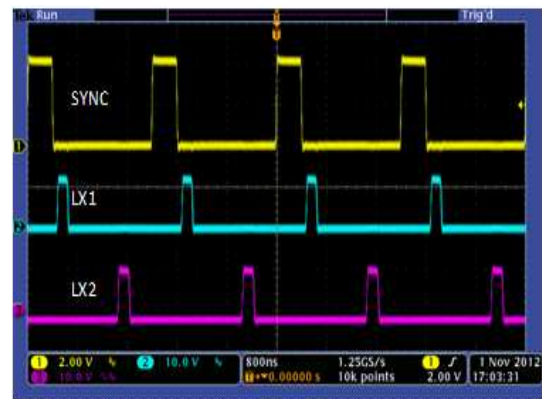
Figure 32. Synchronization at 500 kHz
