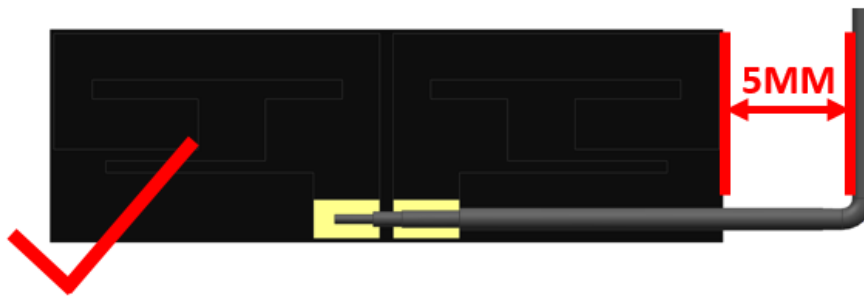
FIGURE 5.2.1 RECOMMENDED CABLE BENDING RANGE
