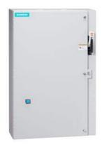
Non-reversing motor starter, Size 4, Three phase full voltage, Solid-state overload relay, OLRelay amp range 50-200A, 550/575 600 50/60HZ coil, Combination type, 200A fusible disconnect, 200A/250V fuse clip, Enclosure NEMA type 1, Indoor general purpose use, Standard width enclosure
