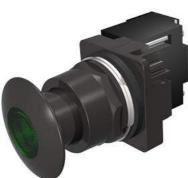
30mm BlackMax, Epoxy Coated Corrosion Resistant Complete Metal Unit Illuminated Push-Pull Operator Transformer type, 240V AC Incandescent Lamp Mushroom Head Cap Small 1 3/4" (44.5 mm) Metal, Black with Green Lens 2 Position Maintained, Pull-to-Release UL Listed, CSA Certified NEMA 1,3,3R,4,4X,12,13 & Automotive Standards
