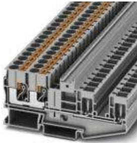
Feed-through terminal block, Connection method: Push-in / plug connection, Cross section: 0.5 mm 2 - 10 mm 2 , AWG: 20 - 8, Width: 8.2 mm, Color: gray, Mounting type: NS 35/7.5, NS 35/15
