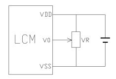
$V_{DD^{\sim}}V_0$ : LCD Driving voltage
