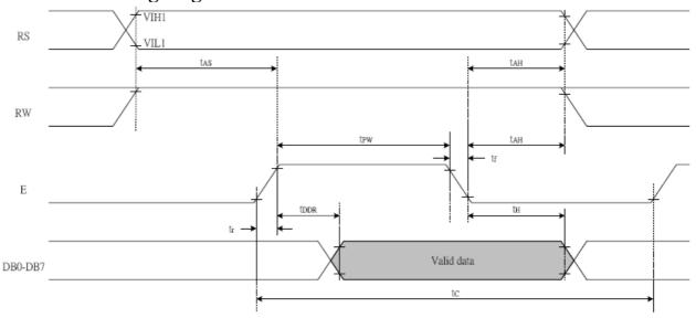
Write cycle (Ta=25°C, VDD=2.7V)
