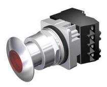
30mm Command/52, Chrome Finish Heavy Duty,Watertight/Oiltight Complete Metal Unit Illuminated Push-Pull Operator Transformer type, 120V AC LED Lamp Mushroom Head Cap Small 1 3/4" (44.5 mm) Metal, Chrome with Red Lens 2 Position Maintained, Pull-to-Release with 1 N.O. - 1 N.C. Heavy Duty Contacts, A600/P600 UL Listed, CSA Certified NEMA 1,3,3R,4,4X,12,13 & Automotive Standards
