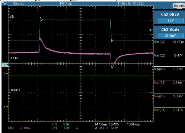
Figure 11. Transient Supply Response V_{OUT} = 3.3\text{ V} , \Delta V = 8\text{ V} to 16.5\text{ V} , 20\text{ mV/div}
