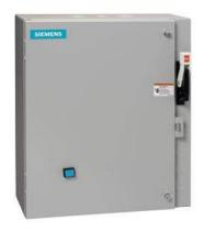
Non-reversing motor starter Size 3 Three phase full voltage Solid-state overload relay OLRelay amp range 25-100A 24VAC 50-60HZ coil Combination type 125Amp circuit breaker Enclosure NEMA type 1 Indoor general purpose use Standard width enclosure
