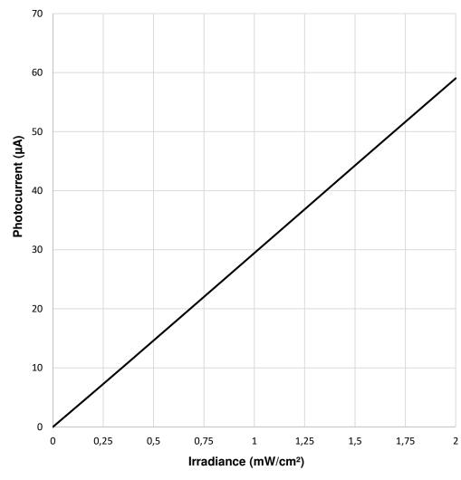
Testcondition: Ee= 0,5 mW/ cm<sup>2</sup>, VR=5V
