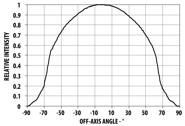
Figure 4. Radiation Pattern for AlInGaP
