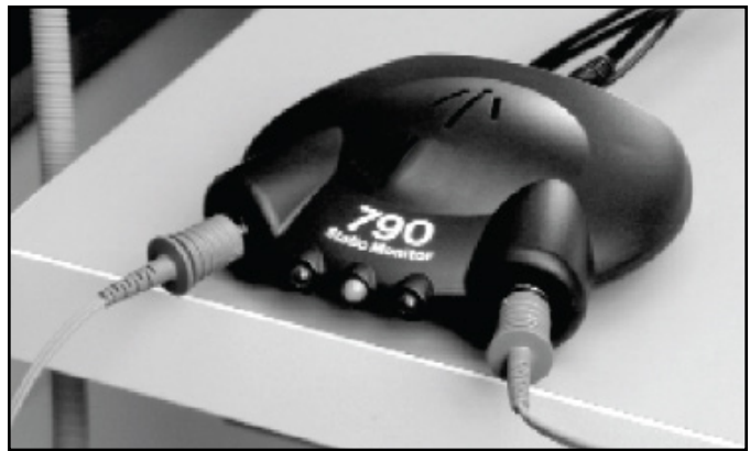
Figure 7. SCS Static Monitor 790 attached to equipment chassis.
