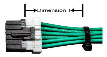
The "T" dimension defines a "free" length of wire, or a length of wire that is not subject to significant bias by external factors such as a wire tie, wire twisting, or other means of bending or deforming of the wires that repositions them from their natural relaxed state or location where they enter the housing. Wires are to be dressed in such a manner
