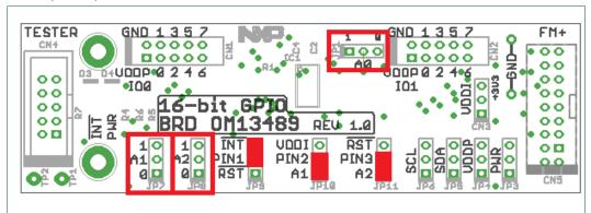
Fig 5. Jumper Configuration for PCA8575, PCA9535A, PCA9535C, PCA9535, PCA9555A, PCA95555, PCA9675, PCAL9535A, PCAL9555A, PCF8575
