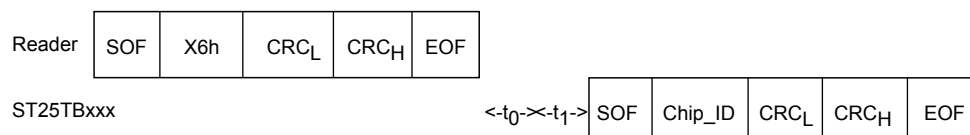
Figure 24. Slot_marker frame exchange between reader and ST25TB512-AT
