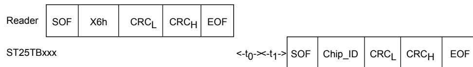
Figure 47. Slot_marker frame exchange between reader and ST25TB512-AT
