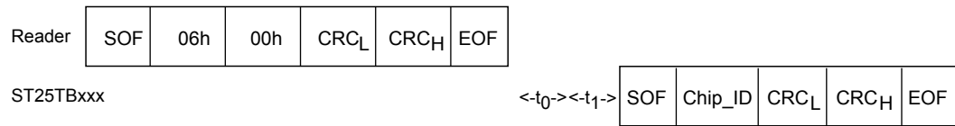
Figure 45. Initiate frame exchange between reader and ST25TB512-AT
