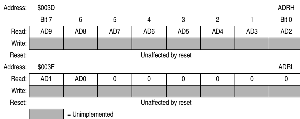
Figure 3-5. ADC Data Register High (ADRH) and Low (ADRL)
