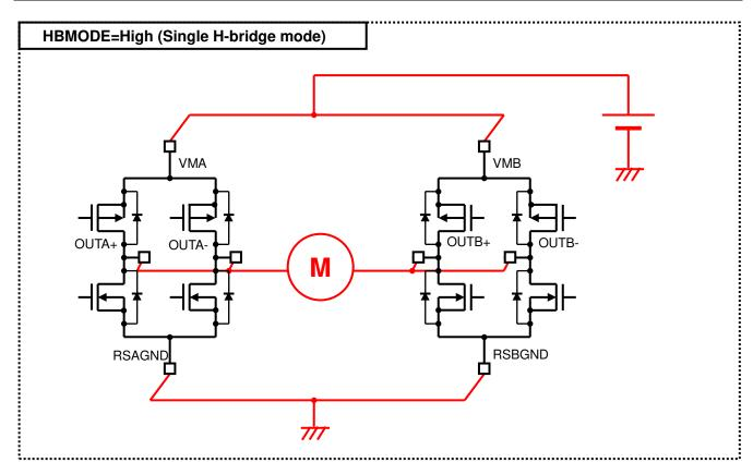
Note: When using the single H-bridge mode, the impedance on the board should be balanced. Also, the power supplies for H-bridges (VMA and VMB), output pins (OUTA+ and OUTA-, OUTB+ and OUTB-), and RSGND pins (RSAGND and RSBGND) should be connected to each other.
