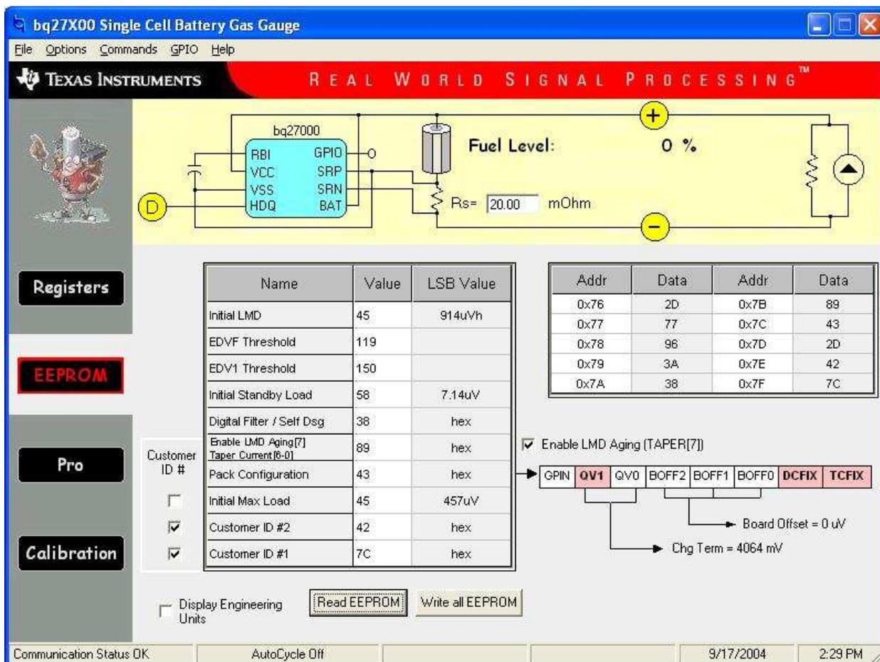
The screenshot shows the 'EEPROM' screen of the 'bq27X00 Single Cell Battery Gas Gauge' software. The interface includes a circuit diagram at the top showing the bq27000 chip connected to a battery and a sense resistor (Rs = 20.00 mOhm). The 'Fuel Level' is displayed as 0%. Below the diagram are several sections:
