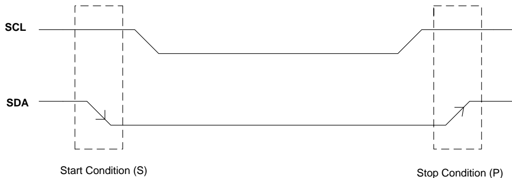
Figure 1. I 2 C Start and Stop Condition
