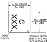
Indicates direction of terminals and start (short) lead. Connect high dv/dt here for lowest EMI.
