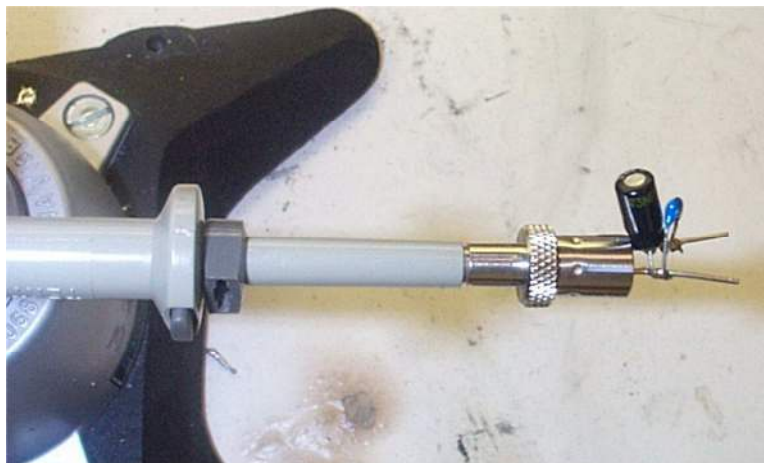
Figure 53 – Oscilloscope Probe with Probe Master ( www.probemaster.com ) 4987A BNC Adapter. (Modified with wires for ripple measurement, and two parallel decoupling capacitors added)
