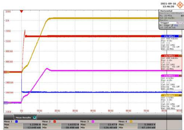
Figure 45 – Output Voltage and Current Waveforms. 265 VAC Input.
