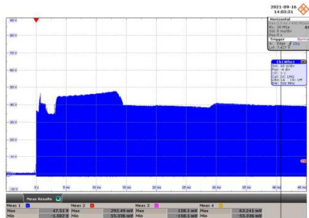
Figure 41 – 5 V FET Voltage Waveforms During Start-Up. 265 VAC Input, Full Load. 5 V_{MAX} = 47.51 V. 5 V SRFET V_{MAX} : 10 V / div. 5 ms / div.
