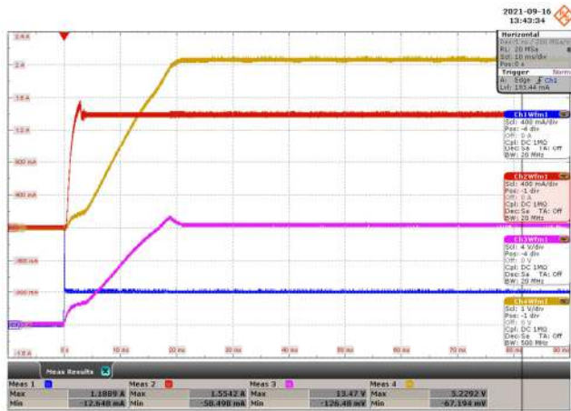
Figure 44 – Output Voltage and Current Waveforms. 85 VAC Input.
