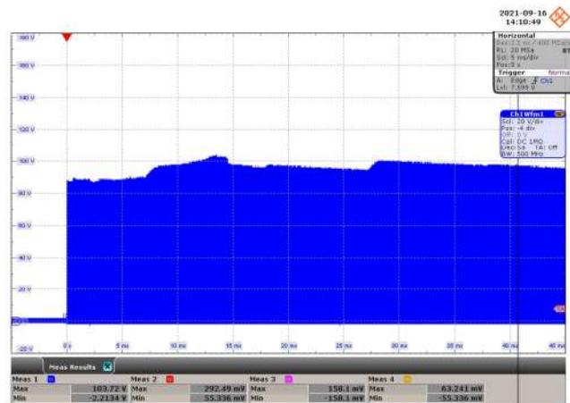
Figure 43 – 5 V Schottky Voltage Waveforms During Start-Up. 265 VAC Input, Full Load. 12 V_{MAX} = 103.72 V. 12 V Schottky V_{MAX} : 20 V / div. 5 ms / div.
