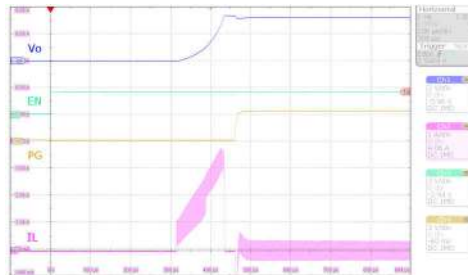
V_I = 4.2\text{ V}, V_O = 3.3\text{ V} MODE = High 100 mΩ resistive load
