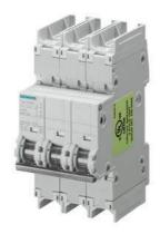
Miniature circuit breaker 240 V 14kA, 3-pole, D, 6 A, D=70 mm according to UL 489  $\,$
