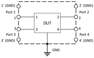
Network Analyzer: Keysight N5242B or equivalent
