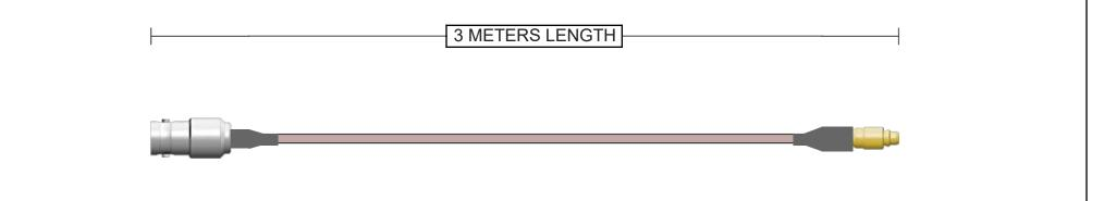
Connector A 112631 BNC Jack Straight Brass Nickel + Heatshrink 50 Ohm RG-178 Continuity/Hi-Pot Connector B 262100 MMCX Plug Straight Brass Gold + Heatshrink
